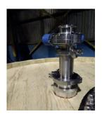
**3" Blow Off Port/CIP Port 3" Clamp connection fitting is**located in the center top of the foeder.
